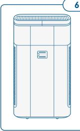
To clean the particle sensor (back of Rediair) lift flap and carefully clean with a cotton swab. This should be done every 2 months or if the LED air indicator consistently shows poor air quality.
