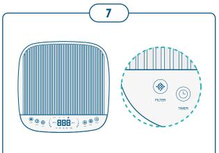
To re-set the pre-filter timer, hold the filter button for 5 seconds until it beeps
