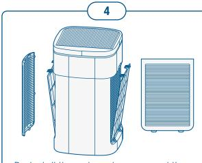
Re-install the external covers and the pre-filters (both sides). **Note:** Ensure external covers are fitted correctly or the Rediair will not power-on.
