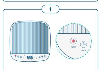
When filter indicator (on the LCD touch control panel) flashes red repeatedly, it is time to clean the pre-filters.
