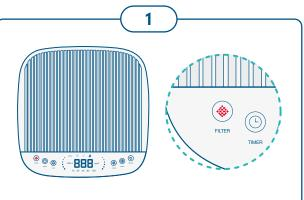
When the filter indicator (on the LCD touch control panel) lights up continuously red OR flashes 5 times and then turns **continuously red** for 5-seconds, it is time to change the all filters.
